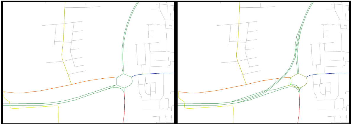
Figure 5-1 Network coding of Sadlers Farm junction improvements
